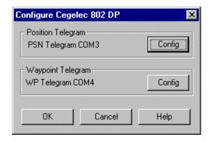
The first item is designating the input/output ports for the interface. In the example above, the output (position) to the Cegelec 802 is via COM 3, while the input/output (Waypoint/Line data) is via COM4. Since the DP system requests, and then receives the Waypoint/Line data from WinFrog, this port operates at full duplex. The Surveyor and DP Operator must ensure that the communication parameters are identical for both the DP System, and this WinFrog COM port.
