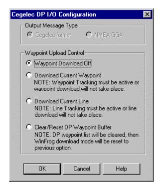
The Output Message Type is not available because only the Cegelec Format position output is available for the Cegelec 802 DP. Note that the Cegelec 901 is also capable of the GGA position output.
