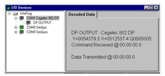
Waypoint and Line data transfer between WinFrog and the Cegelec DP System is configurable via the Cegelec DP I/O Configuration dialog box shown below. This dialog box is accessible after the Cegelec 802 DP device is added, via the Configure > I/O Devices > Configuration command or highlight the Cegelec 802 device in the I/O window, right-click and choose Configure Device.
